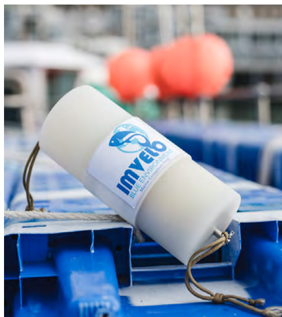
The electronic tension sensor that attaches directly to the BSLs deployed by trawlers in the hake trawl fishery
